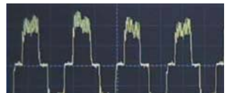
Wave generated by a traditional inverter.
